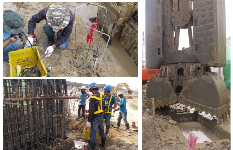
Fig.8 Example of application Measure the lateral movement of pile by inclinometer during Static lateral pile load test.
