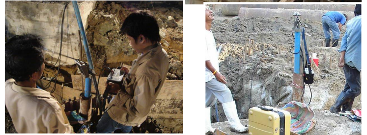
Fig.8 Example of application Measure the lateral movement of pile by inclinometer during Static lateral pile load test.
